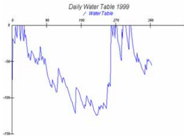
Figure 45. DRAINMOD water table depth plot in centimeters below the surface for 1999
