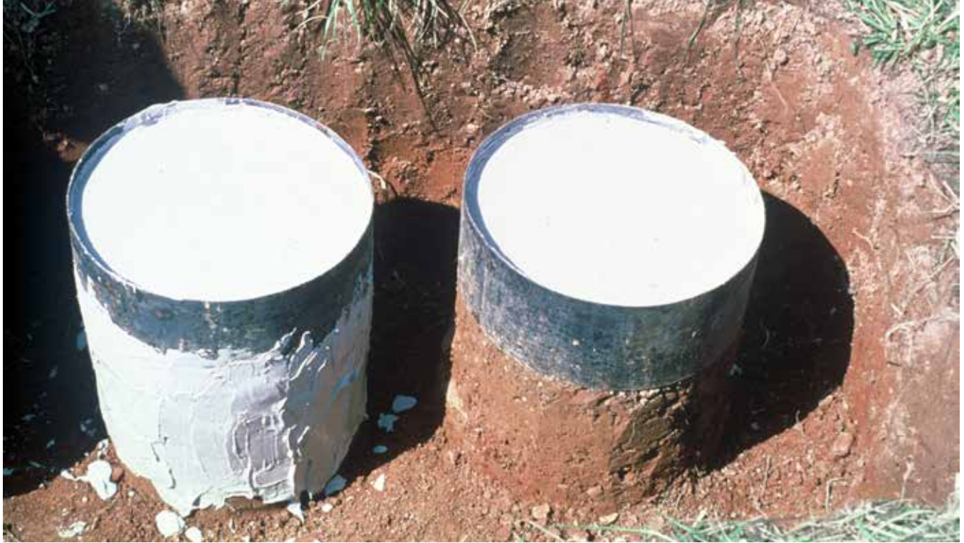
Figure 4. Soil pedestals for in-situ saturated and unsaturated hydraulic conductivity testing, Charlotte, NC
