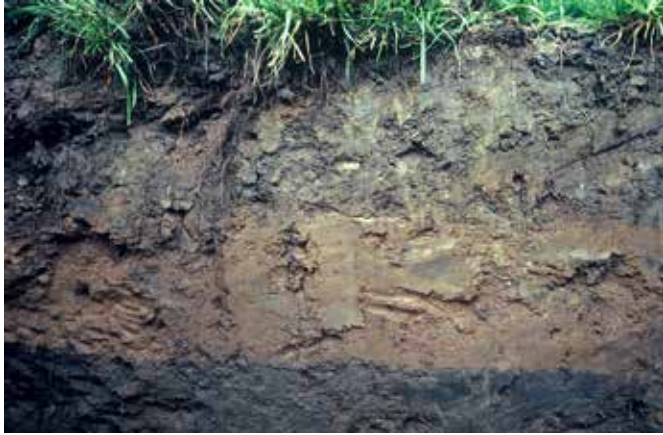
Figure 18. Loamy over Clayey Fill Total Porosity of Clay Layer = 42.3% Macro-Porosity of Clay Layer = 4.1% Bulk Density of Clay Layer = 1.529 National Mall, Washington, DC
