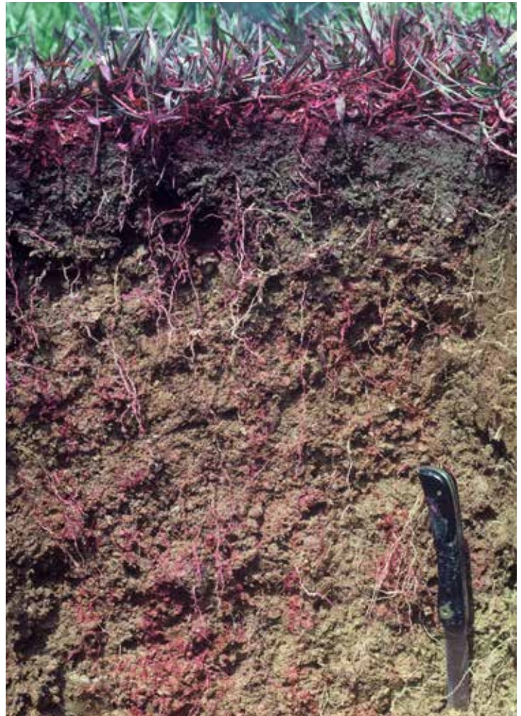
Figure 37. Enhanced infiltration soil profile showing deep rooting.
